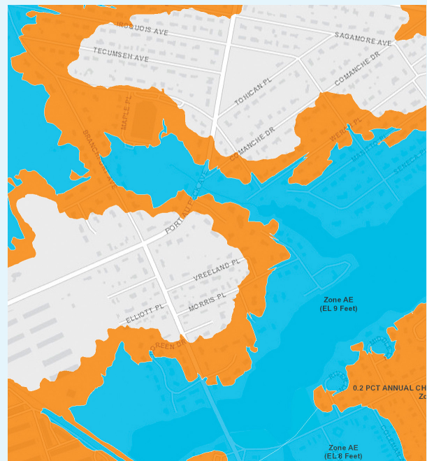
A map of FEMA flood zones generated by NJ FloodMapper delineates 1% (blue) and 0.2% (orange) Annual Chance Flood Hazards, also known as 100-year and 500-year floodplains, in the area around Oceanport, N.J.
